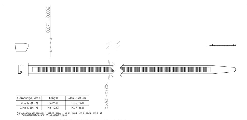
Duct Strap operational temperature is -4F to 185F (-20C to 85C) with a minimum installation temperature of 5F (-15C) per UL 62275.
